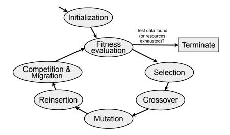
Figure 5: The main steps of a Genetic Algorithm
