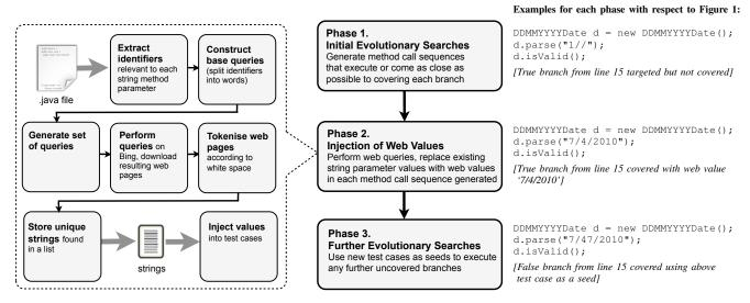
Figure 4. Overview of the steps involved in the test generation process behind Delver, utilising the results of web queries
